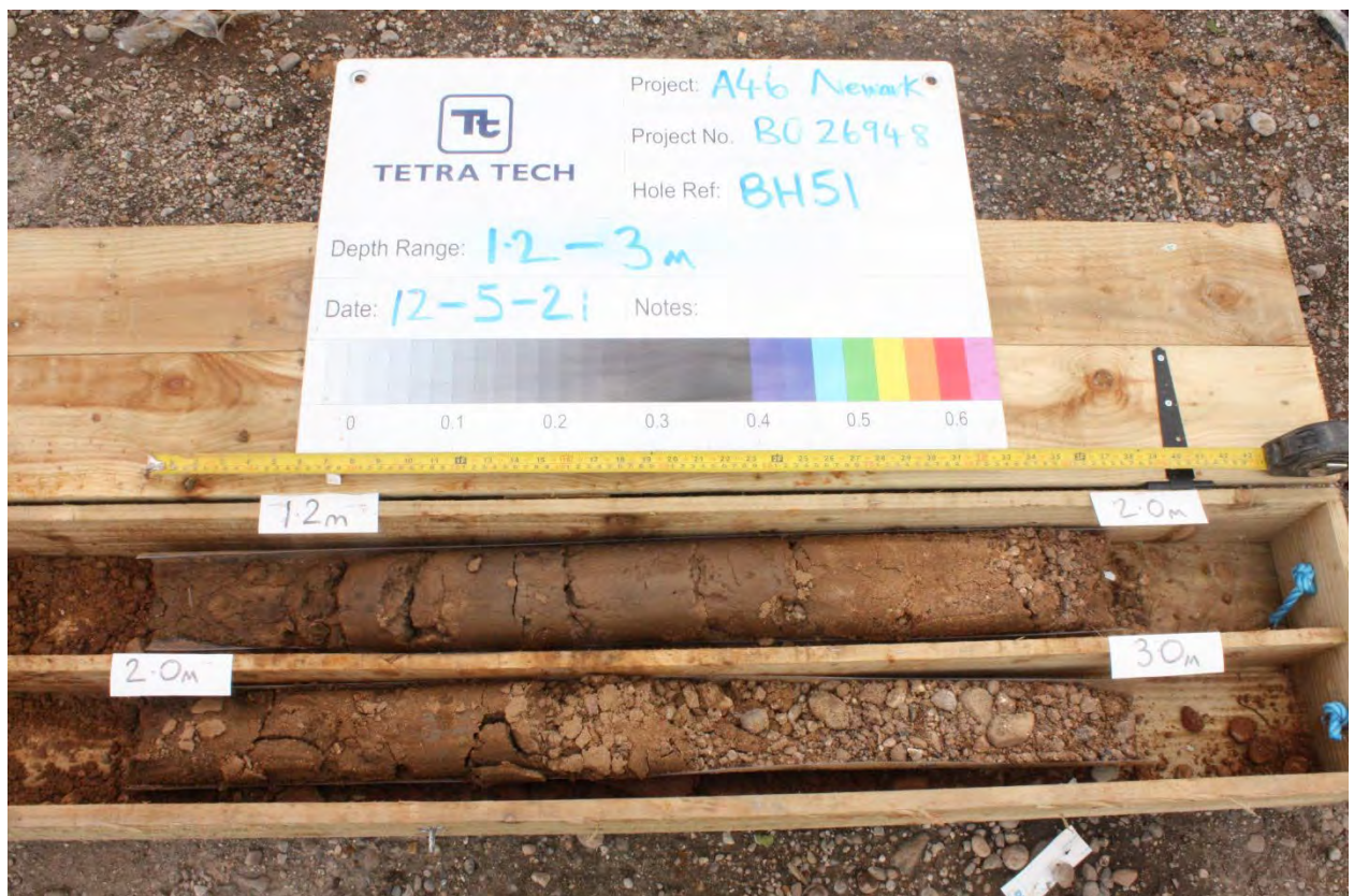
Plate 12: BH51 1.20-3.00m BGL (Sampled 1.35-1.45m BGL; photo shows ex-situ oxidation)
