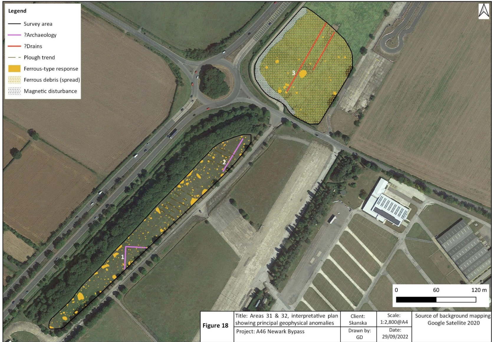
Figure 18: Areas 31 & 32, interpretative plan showing principal geophysical anomalies
