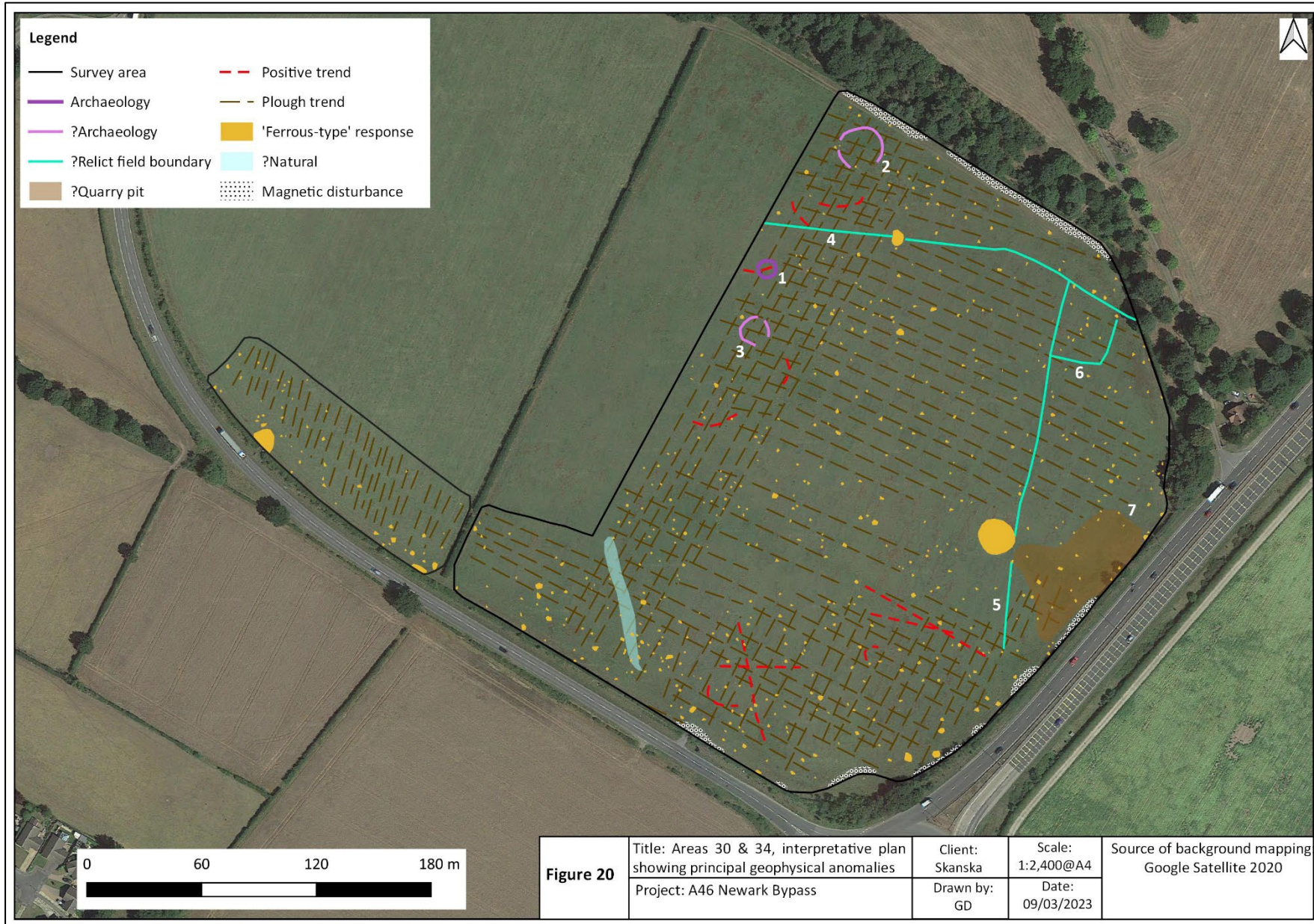
Figure 20: Areas 30 & 34, interpretive plan showing principal geophysical anomalies.
