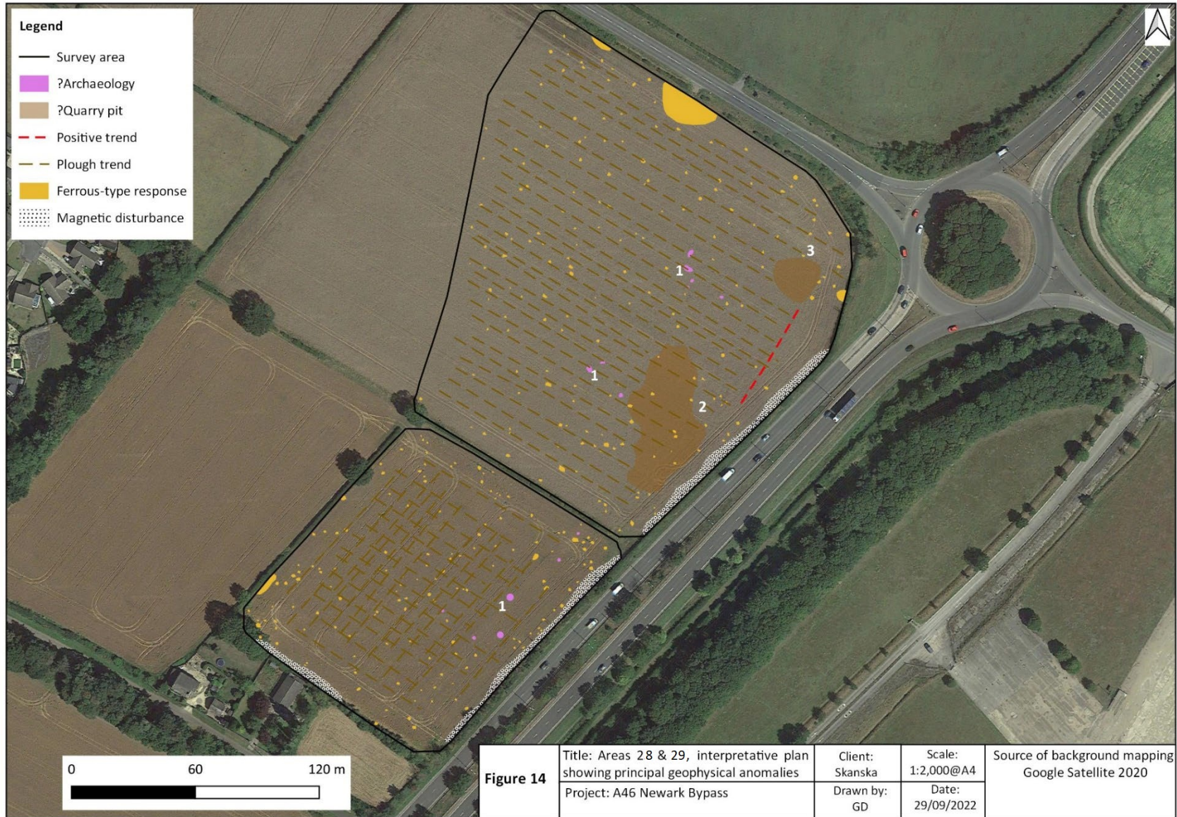
Figure 14: Areas 28 & 29, interpretative plan showing principal geophysical anomalies
