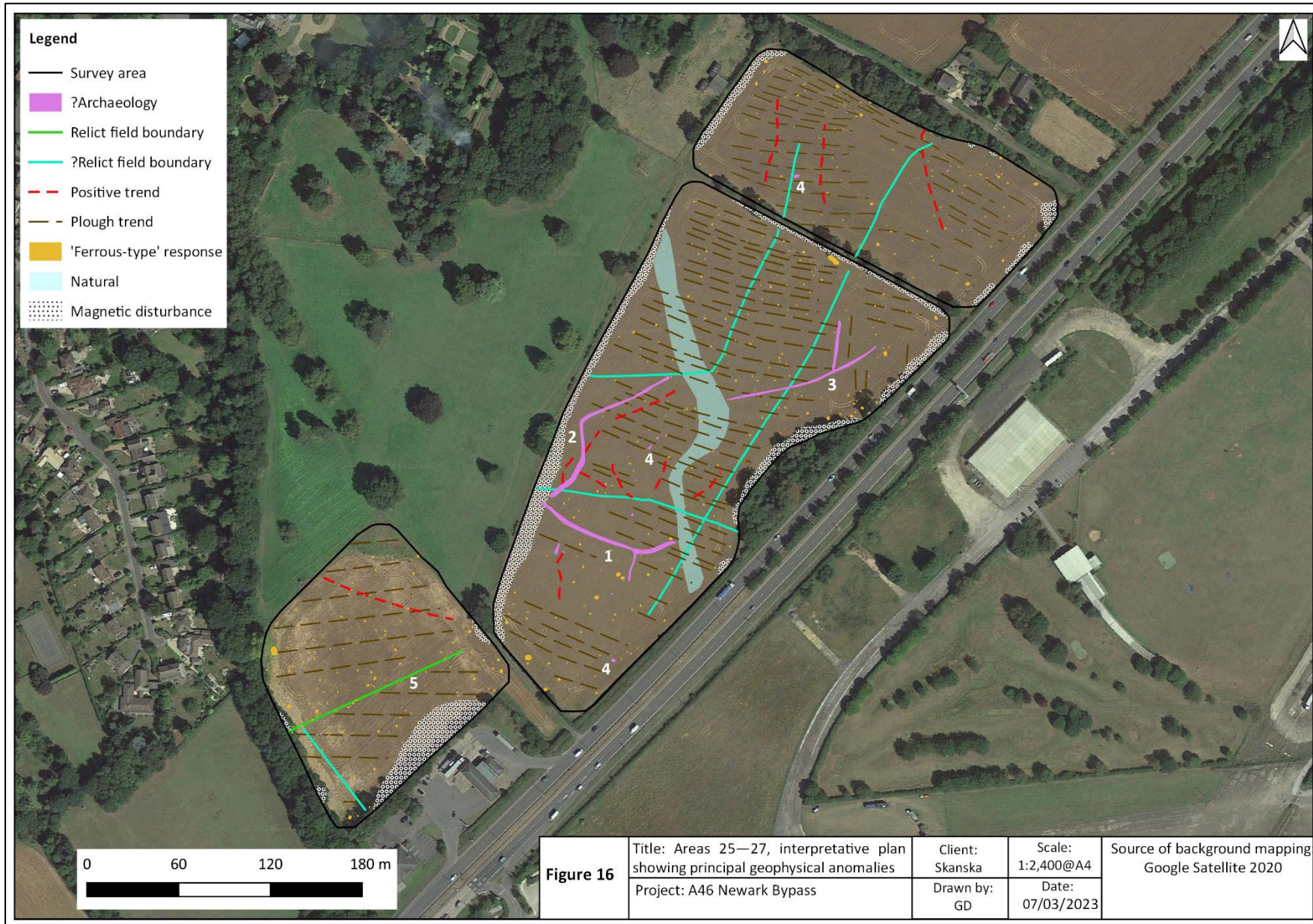
Figure 16: Areas 25—27, interpretive plan showing principal geophysical anomalies.
